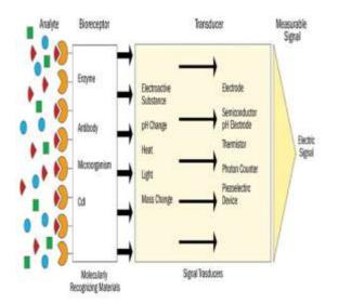
The five principal transducer classes are electrochemical, optical, thermometric, piezoelectric, and magnetic.
