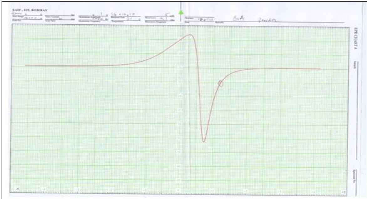
Fig. 4a: EPR Spectrum of Copper
