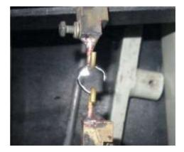
Fig4: Flexibility of cast clasp arm being tested in tensometer
