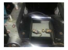
Fig3: Two hooks were custom fabricated to fit the two testing arms of the tensometer to engage the reciprocal and retentive terminal of clasp assembly
