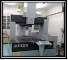
Fig 6. Co – ordinate measuring machine
