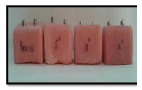
Figure 1: Implant Analogues of Various Angulation (0<sup>0</sup>,50,100,150) Fixed In Resin Blocks
